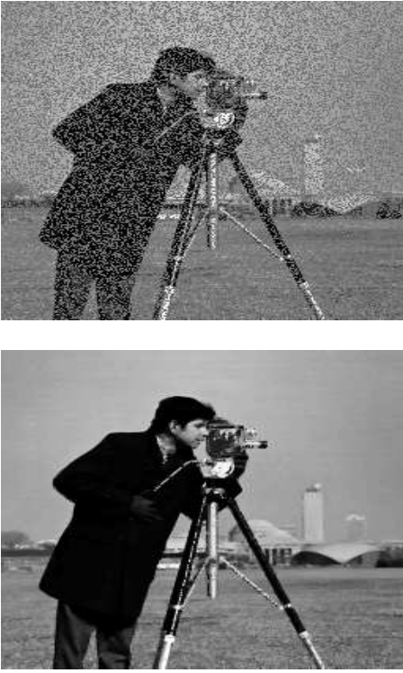
Fig. 9. TV-based image restoration from 40% missing samples (experiment 5); top: observed image; bottom: restored image.
