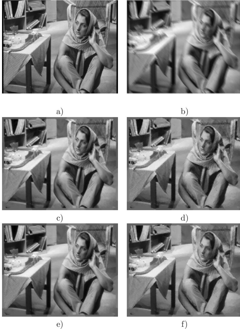
Figure 3.14: “Barbara” image with blur #2. a) Sharp image. b) Blurred image. Next rows: Deblurred images. Left: Without noise. Right: With noise. Second row: Without filter constraints or regularization. Third row: With constraints.
