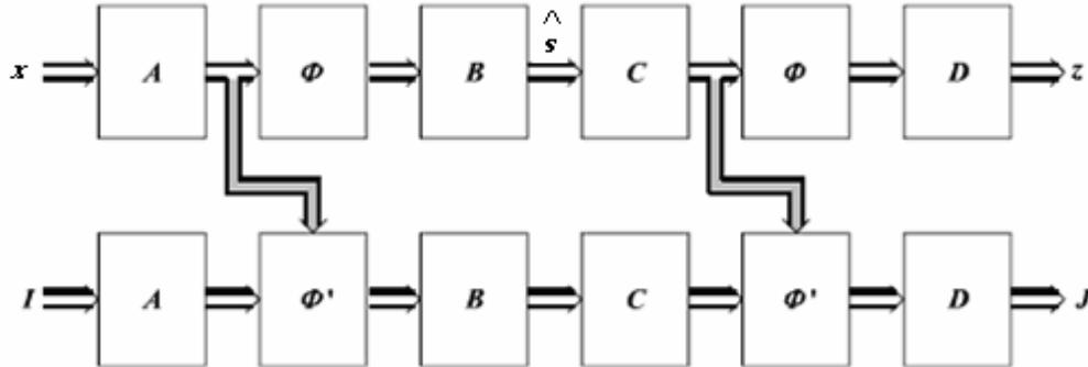
Figure 1.4 – Esquematic representation of the network used by MISEP. The top part corresponds to figure 1.2, drawn in a different way. The lower part, which computes the Jacobian proper, is essentially a linearization of the upper part, but propagates matrices. It has as input the identity matrix, and provides at its output the Jacobian  $\mathbf{J}$ . (Adapted from [21]).
