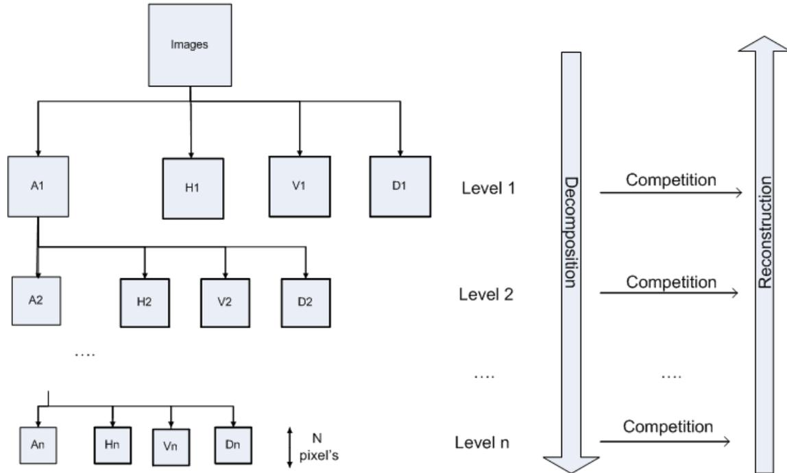
Figure 3.9 - Schematic representation of the second denoising function. On left it is shown the scheme of one image wavelet decomposition in  $n$  levels (the components represented by bold boxes are the ones that will be submitted to the competition). On right it is shown the scheme of the denoising decomposition and the reconstruction of the denoised images.
