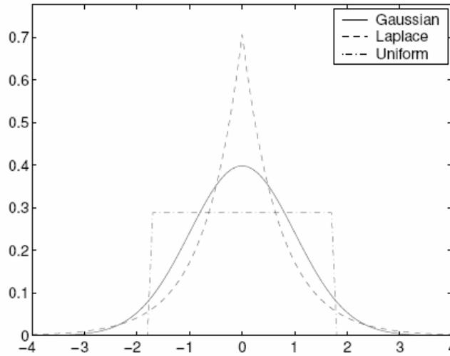
Figure 1.3 – Gaussian, Laplacian (Super-Gaussian) and uniform (Sub-Gaussian) distributions with unit variance. Their kurtosis are 0, 3 and -2 respectively. (from [25]).
