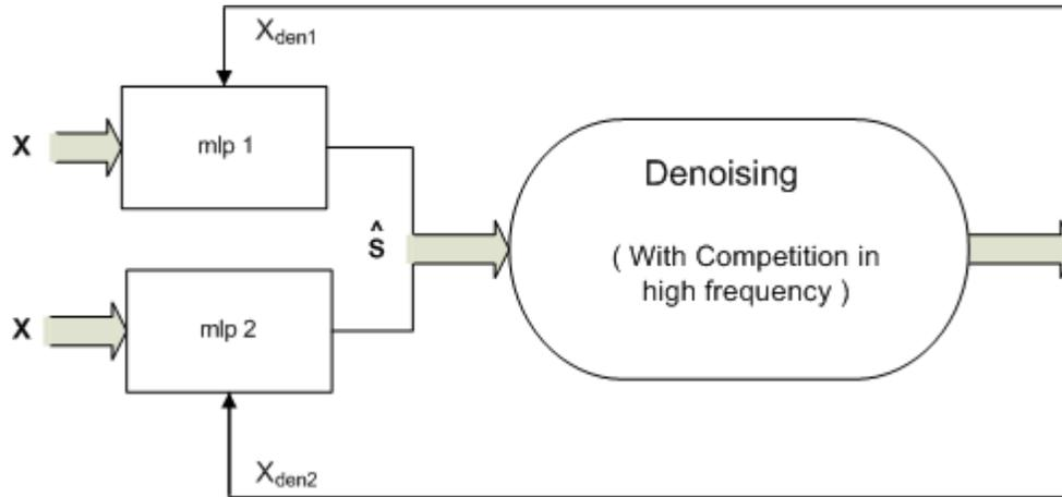
Figure 3.5- Scheme of the proposed nonlinear DSS to separate two nonlinearly mixed images.
