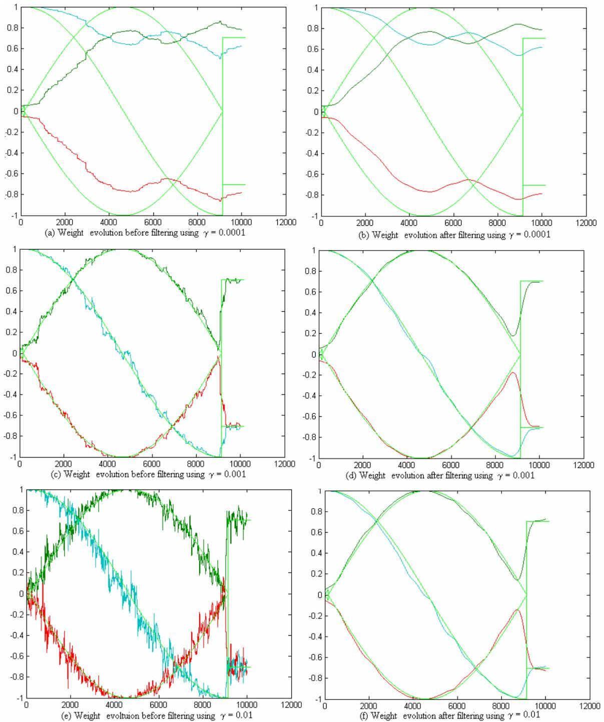
Figure 2.1 - Weight evolution of matrix  $\mathbf{W}$  obtained for the first synthetic mixture. The demixing matrix (inverse of  $\mathbf{M}$ ) is represented by the light green line. The evolution of  $\mathbf{W}_{11}$  (in dark blue) is overlapped by the evolution of  $\mathbf{W}_{22}$  (in light blue).
