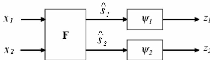
Figure 1.2 – Schematic representation of the network used by *Infomax* in order to separate two sources. The **F** bloc performs ICA and  $\hat{S}_i$  are the extracted components.  $\psi$  's are the auxiliary blocs of training ( adapted from [21] ).
