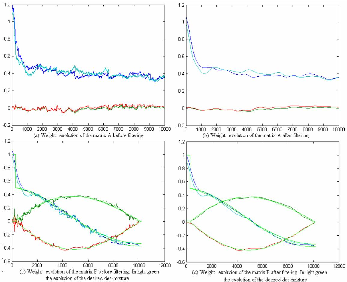
Figure 2.2 - Results obtained for the second synthetic mixture. The value of  $\gamma$  was 0.002 and  $\beta$  was 0.002. The demixing matrix (inverse of  $\mathbf{M}$ ) is represented by the light green line.
