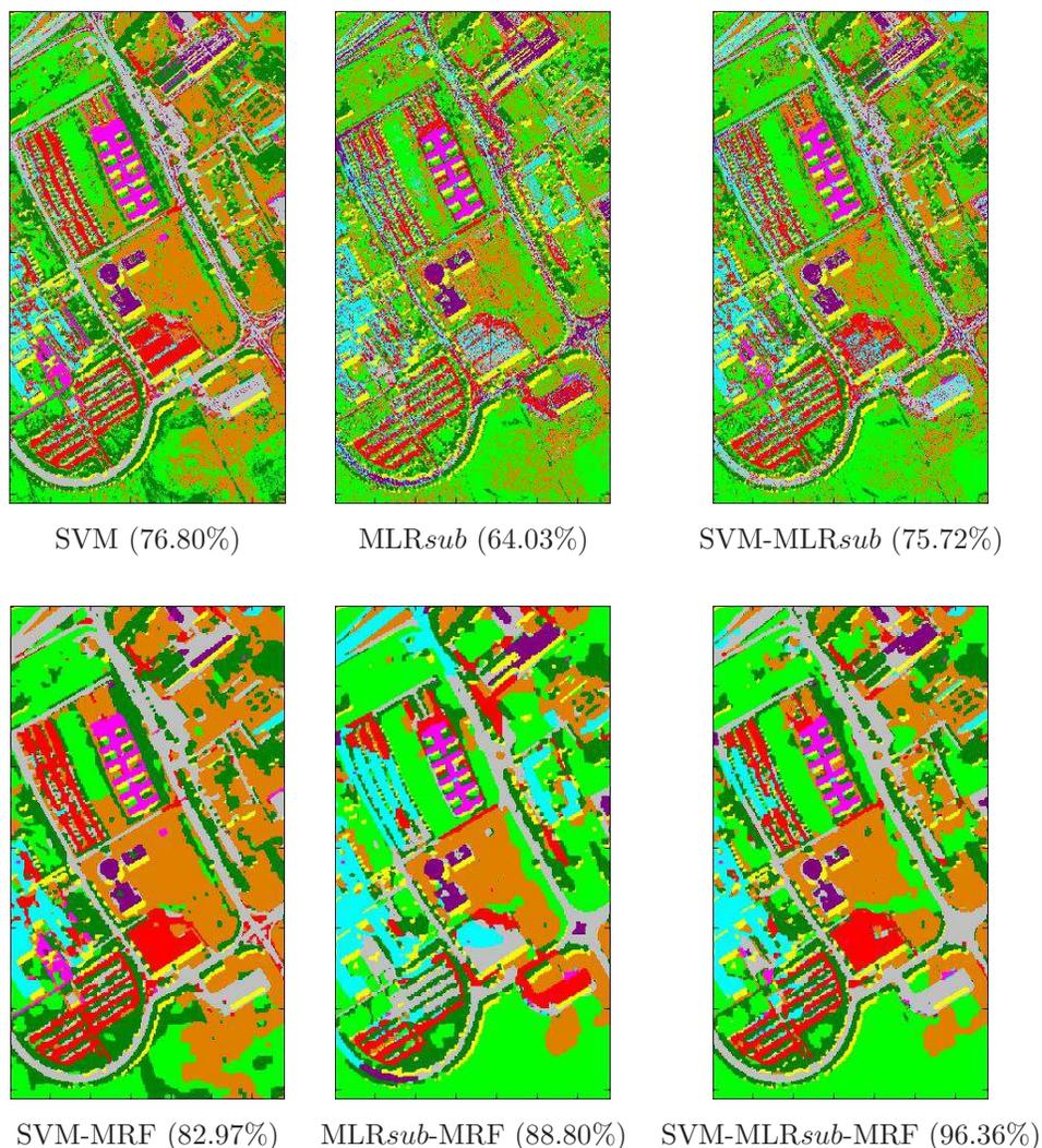
Figure 2.8: Classification results and overall classification accuracies (in the parentheses) obtained by different methods for the ROSIS Pavia University data set.
