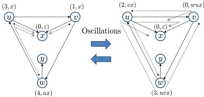
Fig. 3. Destination is  $x$ . Couplets of the routes elected by the nodes are indicated next to them. As a visualization aid, the dashed paths mark the path-complement of couplets. The routing vector protocol oscillates indefinitely between the routing state depicted on the left-hand side and the routing state depicted on the right-hand side.
