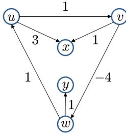
Fig. 1. Links point in the direction of data-packet flow. The length of a link is indicated next to it. Cycle  $uvwu$  has a negative length of  $-2$ .
