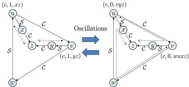
Fig. 6. Inter-domain routing policies involving customers, providers, and siblings. Destination is  $z$ . Attributes of elected routes at ASs  $u$  and  $v$  are indicated next to these nodes. Dashed paths mark the values of AS-PATH. BGP oscillates indefinitely between the routing state depicted on the left-hand side and the routing state depicted on the right-hand side.
