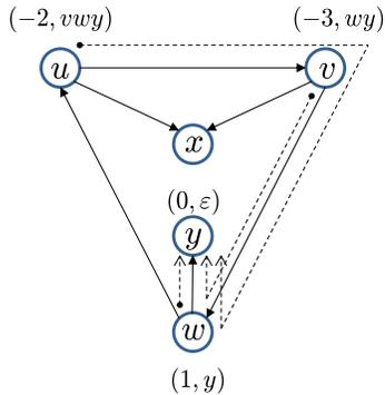
Fig. 2. Destination is  $y$ . Couplets of the routes elected by the nodes in the stable state are indicated next to them. As a visualization aid, the dashed paths mark the path-complement of couplets. The stable state does not contain a forwarding loop.
