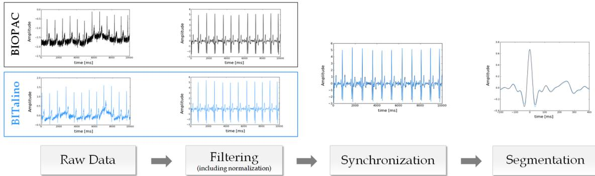
Figure 1: Block diagram of the pre-processing steps we have performed, to compare the signals acquired from both devices. The curves plotted in black were acquired using the BIOPAC while the blue ones with the BITalino
