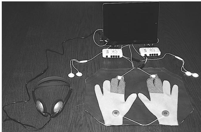
Figure 1: Biosignal acquisition setup.
