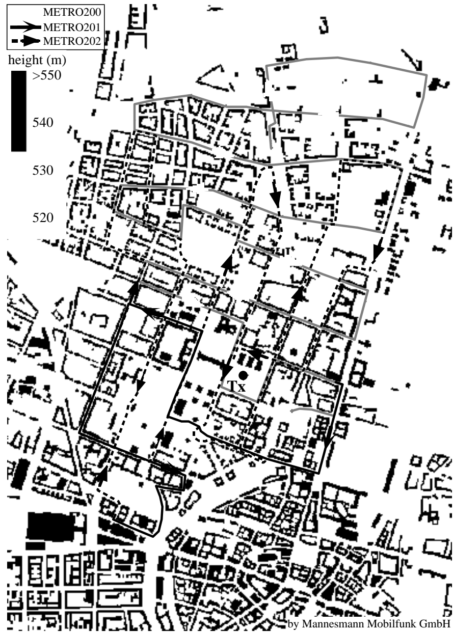
Fig. 4.5.2 Munich test site with measurement routes (~ 25 km) and transmitter location; terrain height is grey scaled.
