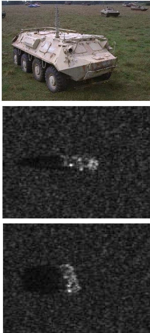
Figure 3.8: Visible (top) and X-Band (middle and bottom) images of the BTR 60 transport vehicle (data from the MSTAR data public collection). Aspect angles of the middle and bottom images are nearly 0^\circ and 90^\circ , respectively.
